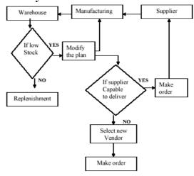
Fig. 4. Task reference model for low inventory in the warehouse
