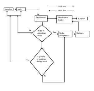
Fig. 5. Task reference model for inventory replenishment (Order management)in the warehouse
